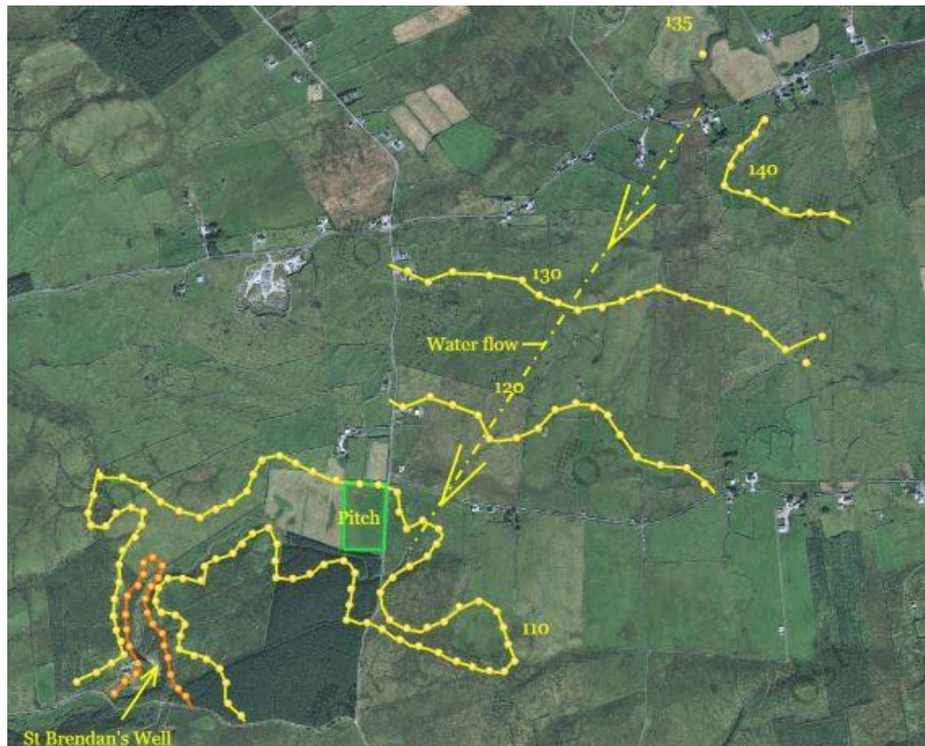
Contours relating to surface drainage toward and beyond the pitch
